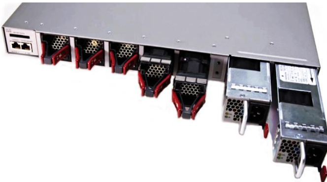
Figure 6. Redundant Fan and Power Supply
