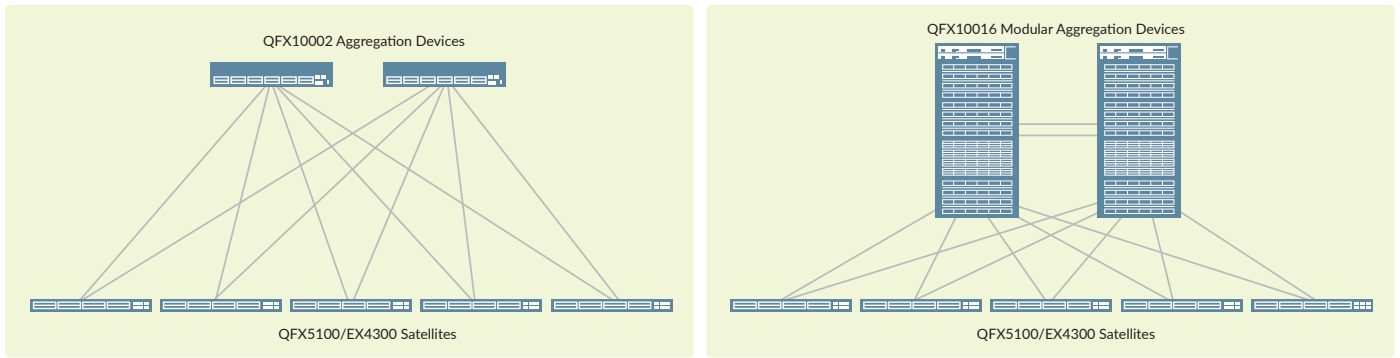
Figure 2: Junos Fusion deployments using QFX1000 switches as Aggregation devices and EX4300 and QFX5100 switches as Satellite devices.
