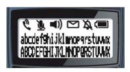
The handset LCD consists of three rows. The top row consists of six icons while the remaining two rows consist of 24 alphanumeric characters.
