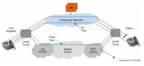
The following figure illustrates how TEHO works:
