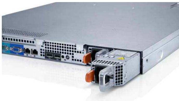
Figure 7. 350W power supply unit
