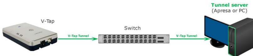
A connection between V-Tap and Apresa or PC software is needed to get the recorded data automatically into a user accessible database.
