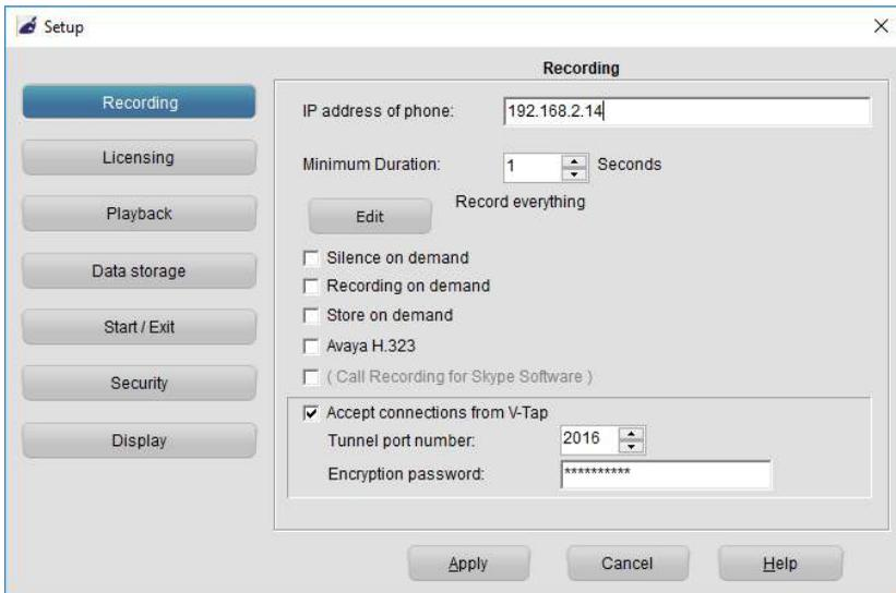
**NOTE1:** The PC's IP address is the "Tunnel Server Address" in the V-Tap.
