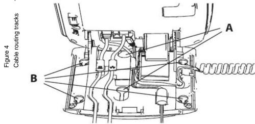
**Step 8: Wall-mount your phone (optional).** Your Avaya 1140E IP Deskphone can be mounted either by: (Method A) using the mounting holes on the bottom of the phone stand, or (Method B) using a traditional style wall-mount box with RJ-45 connector and 15-cm (6-inch) CAT5e cable (not provided).
