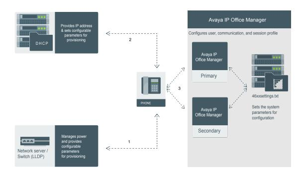
Figure 4: Setup in IP Office environment
