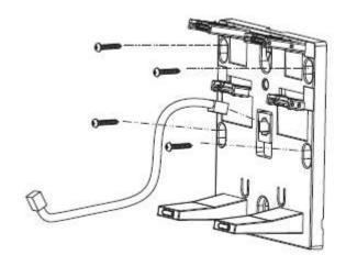
• If there is a pre-installed wall plate, place the wall mount bracket over the wall plate. In this case, you do not need the screws.
